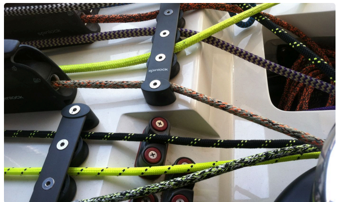
Rigging detail: running lines led through Spinlock clutches.
