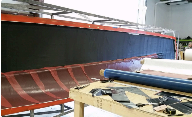
Laying prepreg into the hull mold, August 2016.
